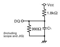
Fig.1 Output load
